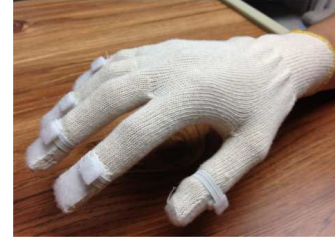
Fig. 7. Glove used to keep thimbles on fingertips.
