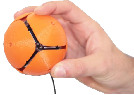
Fig. 1. The Patched Intrinsic Tactile Object with spherical shape, grasped by a human hand.
