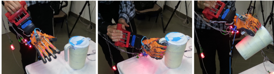
FIGURE 1. Pictures taken during the recording of the jug sub-dataset. The operator drives the SoftHand towards the object, then grasps and lifts it, while sensor data is being recorded.
