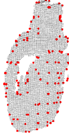
Fig. 4. Keypoints (in red) extracted from the point cloud of a bottle
