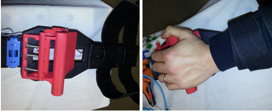
FIGURE 4. The handle for SoftHand without (left) and with (right) the operator's arm. The lever to close the SoftHand is located where the operator's hand should rest.
