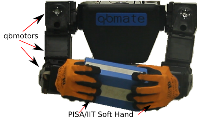
Fig. 1. The Motion planning method presented in this paper is developed for systems with compliance either in their structure or via the control loop. In this case the bimanual system includes the compliance in the qbmotors [9] composing the structure which is combined with mechanically embedded compliance of the PISA/IIT SoftHands [10]. In this paper we consider that all compliance is in the contact points.
