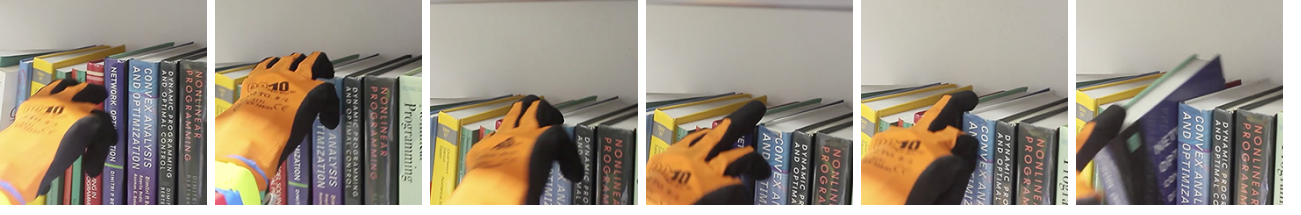
Fig. 4. A person with the arm-mounted SoftHand can seamlessly execute also difficult manipulation tasks which involve combined interactions between hand, object and the environment.
