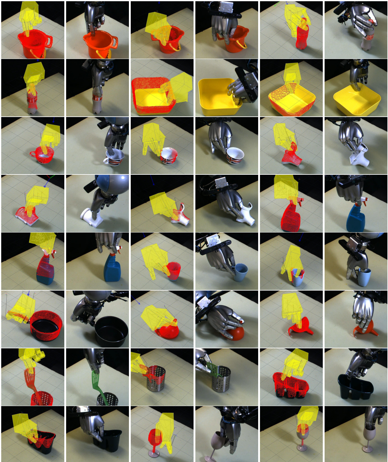
Fig. 9. The test objects with a visualisation of some of the successful grasps. Each grasp is shown by a pair of images, with the visualisation of the planned grasp and the obtained point cloud on the left, and the actual grasp execution on the right. Those from the 7 view and 1 view conditions can easily be distinguished by the proportion of the object covered by the recovered point cloud.
