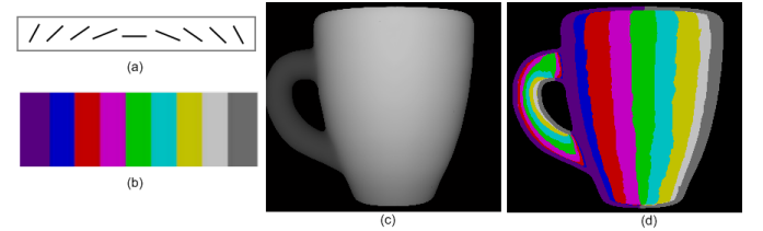
Fig. 3. (a) Pre-defined first layer parts. (b): Color coding of the first layer parts. (c): Range image of the mug. (d): Encoding of the mug with first layer parts.
